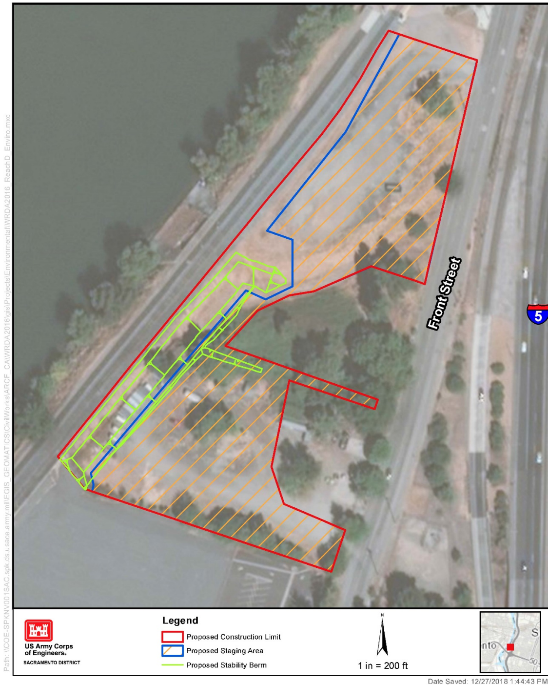
Figure 3. Alternative 2 – Drained Stability Berm Construction (Proposed Action).
